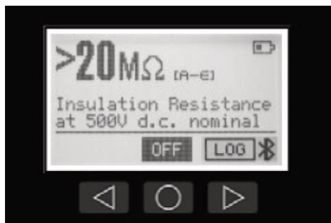
Insulation Resistance Test
