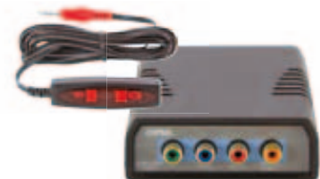
2. Infrared remote command reaches the balun via the IR target
